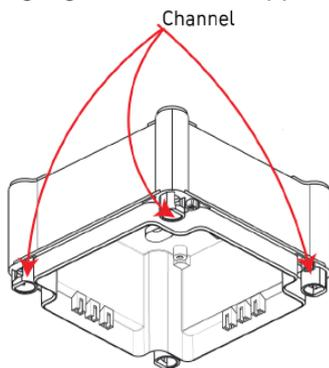
4. Install the gland in position. Make sure it is installed properly to retain IP rating.
